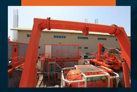
PETRODIVE Saturation diving system (PDS1) is capable of handling six divers in saturation.
